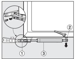
■ Open the hinges, and loosen the screw in mounting ①.
